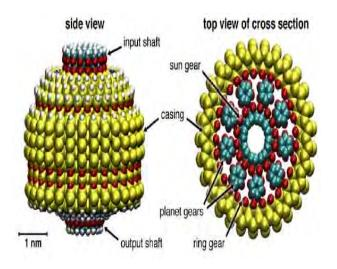
Figure 3. A molecular planetary gear [24]
